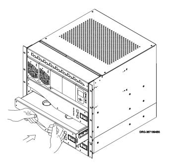
To confirm the battery tray is properly latched, pull gently on the recessed handle. The battery tray should not slide out.
