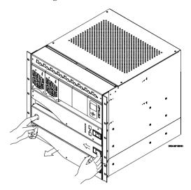
**2** Pull the blanking tray out, until it reaches the end-stops.
