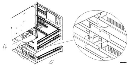
**2** Ensure that the bus bars of the extended battery chassis are positioned behind the bus bars of the NES.
