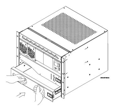
To confirm the blanking tray is properly latched, pull gently. The blanking tray should not slide out.
