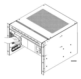
**2** Confirm that the rectifier is properly inserted. The rectifier should not slide out easily.
