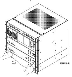
**2** Pull the battery tray out until it reaches the end stops, as shown below.
