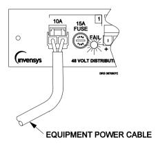
Details about replacing a DC distribution fuse can be found in Chapter 6.
