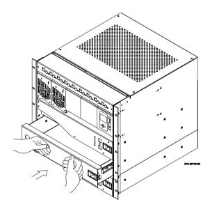
To confirm the blanking tray is properly latched, pull gently. The blanking tray should not slide out.
