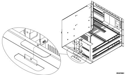
2 Screw the cover plate to the extended battery chassis that you will be mounting last (the bottom-most), as shown below.
